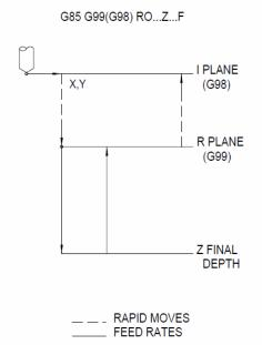
Figure 4-15 G85-Bore In, Bore Out
