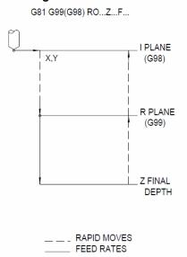
Figure 4-9 Spot Drilling
