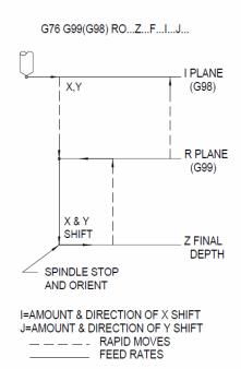
Figure 4-8 Fine Boring Using I, J
