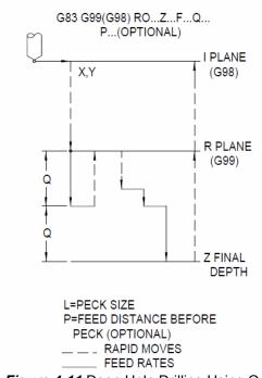
Figure 4-11 Deep Hole Drilling Using Q
