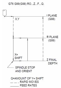
Figure 4-7 Fine Boring Using Q
