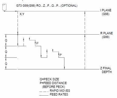
Figure 4-2 Peck Drilling Using Q
