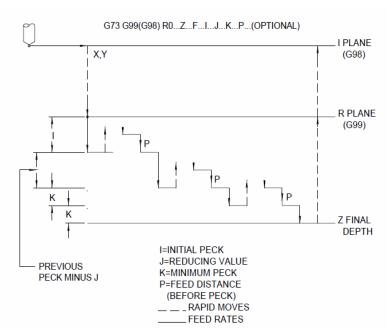
Figure 4-3 Peck Drilling Using I, J, K
