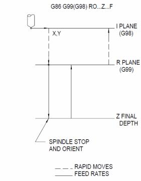
Figure 4-16 G86-Bore In, Spindle Off, Rapid Out
