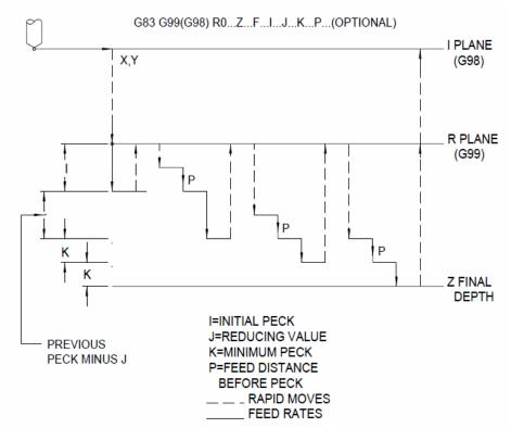
Figure 4-12 Deep Hole Drilling Using I, J, K
